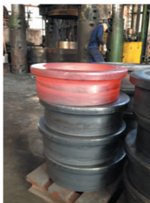
Hot forging of 20" CuNi stub ends
