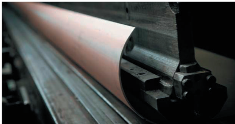
U-BEND PRESS forming CuNi plate into pipe
