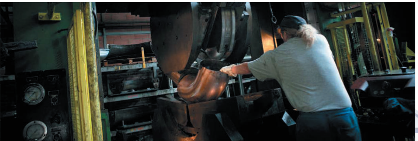
Cold forming CuNi elbows from seamless pipes
