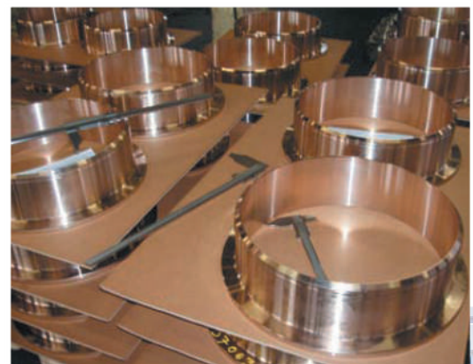
CuNi Inner flanges final inspection
