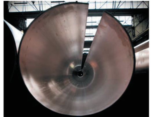
3 ROLLS CuNi pipe forming
