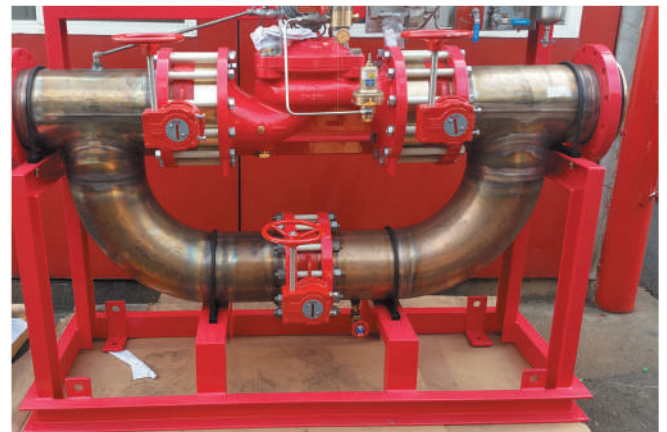
Fire Fighting piping skid 90/10 CuNi
