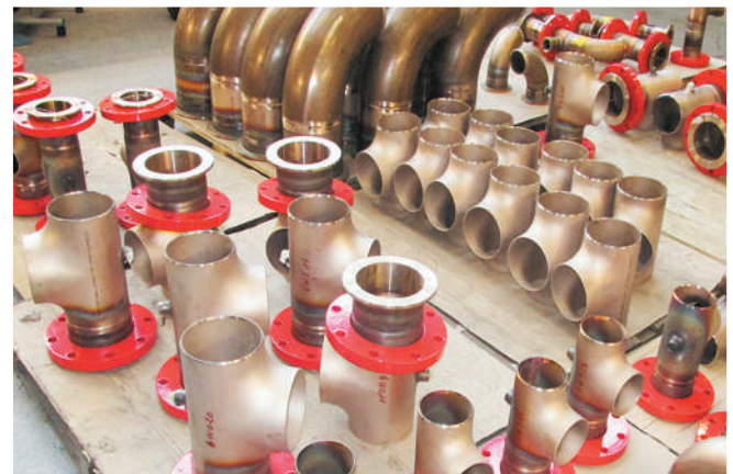
90/10 CuNi piping spools
